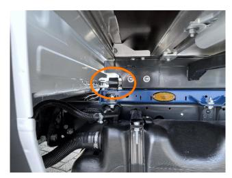
• After coupling, check whether the left and right guide pins behind the vehicle cab are correctly positioned in their guide rails
