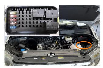
• The IBS fuses are located in the fuse box of the IBS computer in the vehicle as shown
