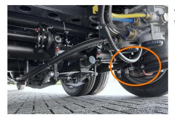
• Check the nuts on the U-bolts. Tightening torque **550 Nm**
