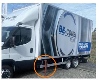
• After coupling the vehicle and trailer, check the removal of the left and right trailer support
