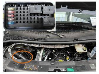
• The IBS fuses are located in the fuse box of the IBS computer in the vehicle as shown
