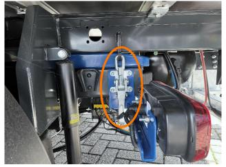
• Check the left and right rear of the trailer for correct positioning of hook clamps
