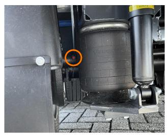
• Position of grease nipple on anchor plate, left and right sides
