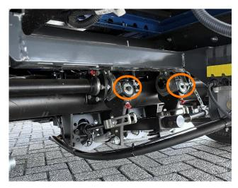
• Check if the distance between the automatic slack adjusters is parallel.
