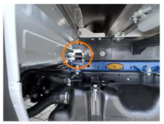
• Lubricate the pin on the front left and right sides of the fifth wheel with ceramic grease
