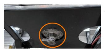
• Check the kingpin bolt connection. Tightening torque **130 Nm**
