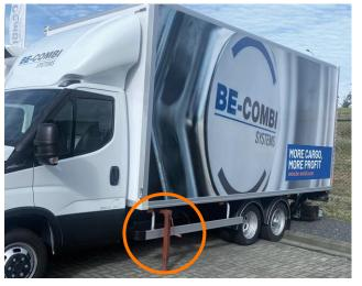
• After coupling the vehicle and trailer, check the removal of the left and right trailer support
