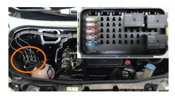
• The IBS fuses are located in the fuse box of the IBS computer in the vehicle as shown
