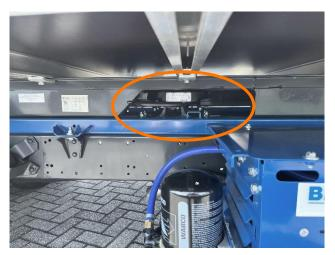
Check that the fifth wheel lever on the passenger side is fully retracted and secured by the locking lever
