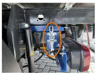
• Check the left and right rear of the trailer for correct positioning of hook clamps
