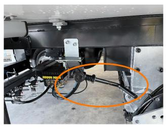
• Check if the trailer parking brake is released, operated by the spindle on the driver's side
