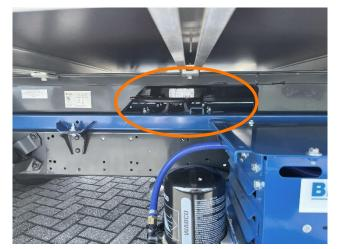
• Check that the fifth wheel lever on the passenger side is fully retracted and secured by the locking lever
