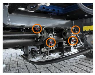
• Lubricate the axle with high pressure grease (EP)
