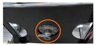
• Check the kingpin bolt connection. Tightening torque **130 Nm**
