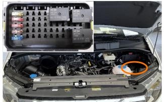
• The IBS fuses are located in the fuse box of the IBS computer in the vehicle as shown
