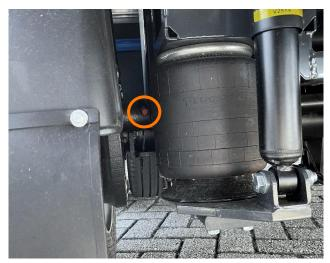
• Position of grease nipple on anchor plate, left and right sides
