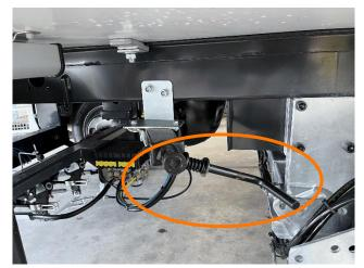
• Check if the trailer parking brake is released, operated by the spindle on the driver's side
