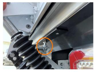
• Screw 2x support bolt against bottom stop and fasten it
