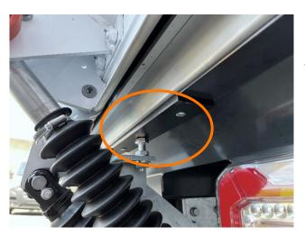
• **CAUTION!** Place 2x stop plate on rear light panel hole pattern with monobolts in case of tail lift assembly
