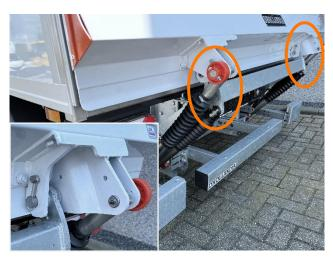
• Mount valve at 4x pivot point and fasten with corresponding bolt
