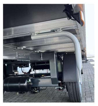
• If necessary, install side shield brackets as shown
