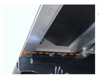
Measurement point front end front side of box
