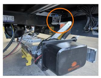
• Lock horizontally by means of 2x glue clamp as shown
